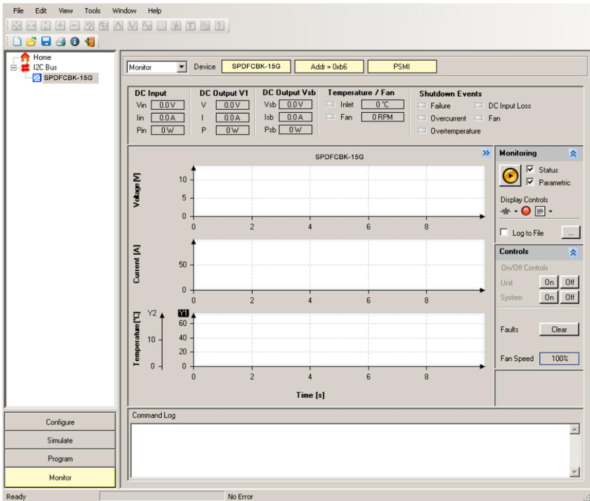
The monitoring screen also allows to enable the hot-standby mode on the power supply. The mode status is monitored and by changing the load current it can be monitored when the power supply is being disabled for further energy savings. This obviously requires 2 power supplies being operated as a redundant system (like the evaluation kit).
