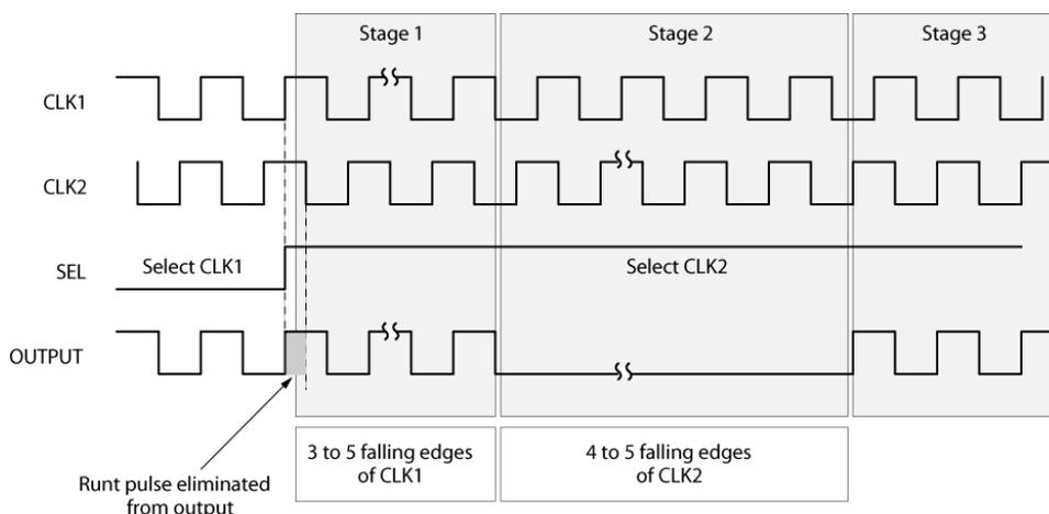
Figure 2. Timing Diagram 1
