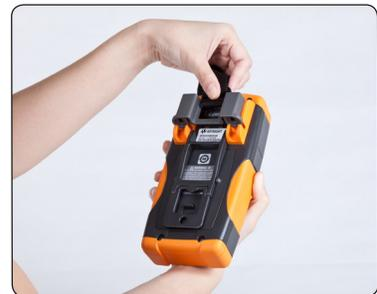
3) Snap the adapter tightly to secure the connection.
