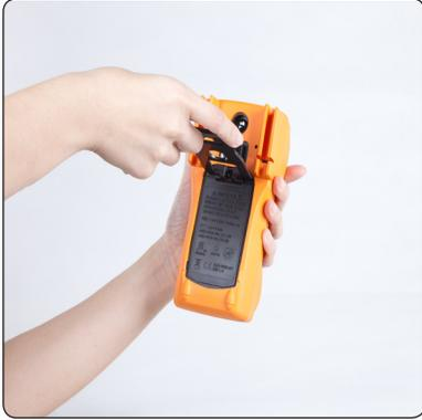
2) Flip the stand over so that the stand's inner surface is facing the meter's rear.
