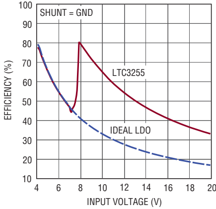
3.3V OUT Efficiency vs Input Voltage at 50mA Load
