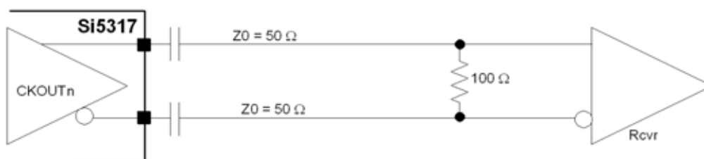
Figure 11. Typical Differential Output Circuit
