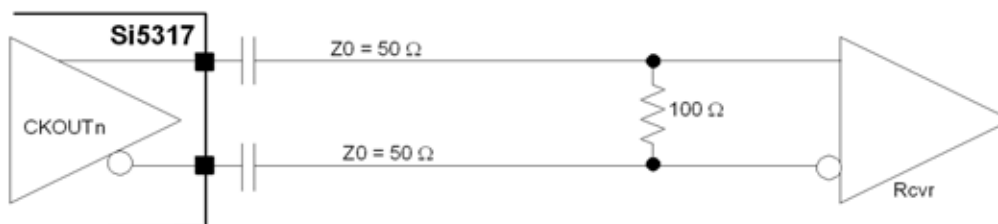
Figure 11. Typical Differential Output Circuit
