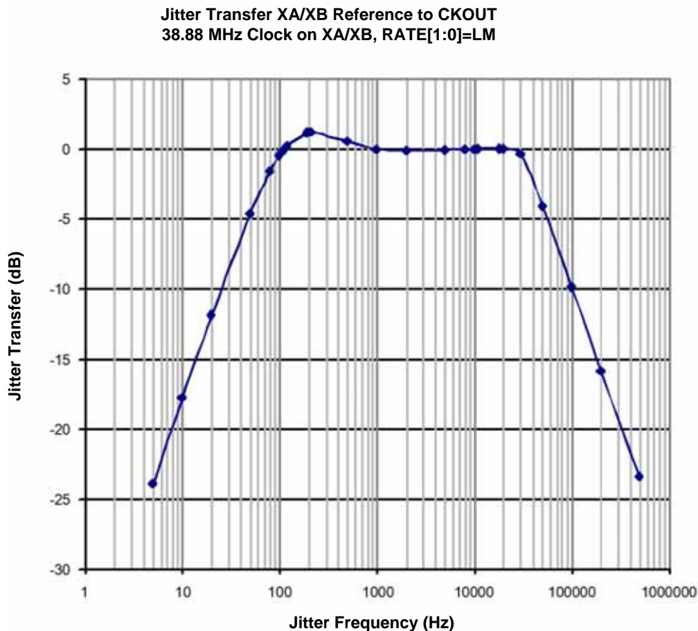
Figure 17. Typical XA-XB Jitter Transfer Function
