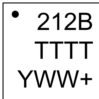
Figure 6.3. QFN20 Package Marking
