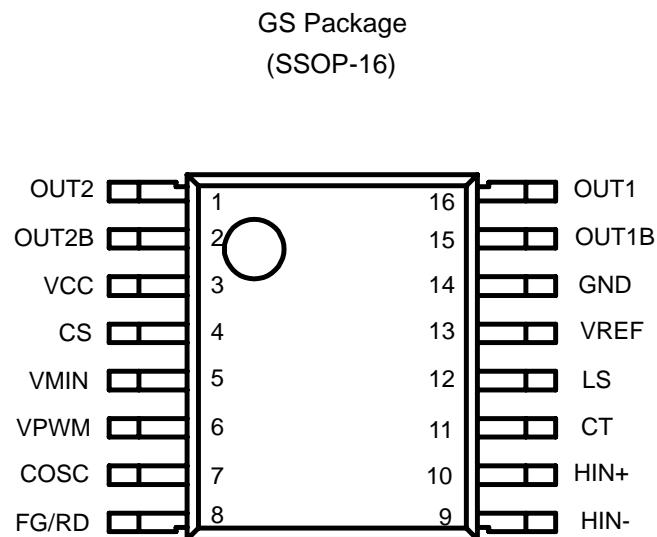
Figure 2. Pin Configuration of AM4967
