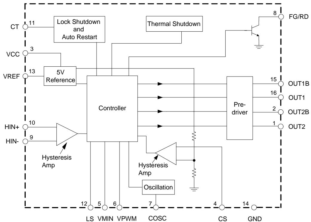
Figure 3. Functional Block Diagram of AM4967
