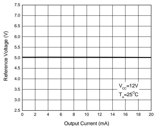
Figure 7. Reference Voltage vs. Output Current
