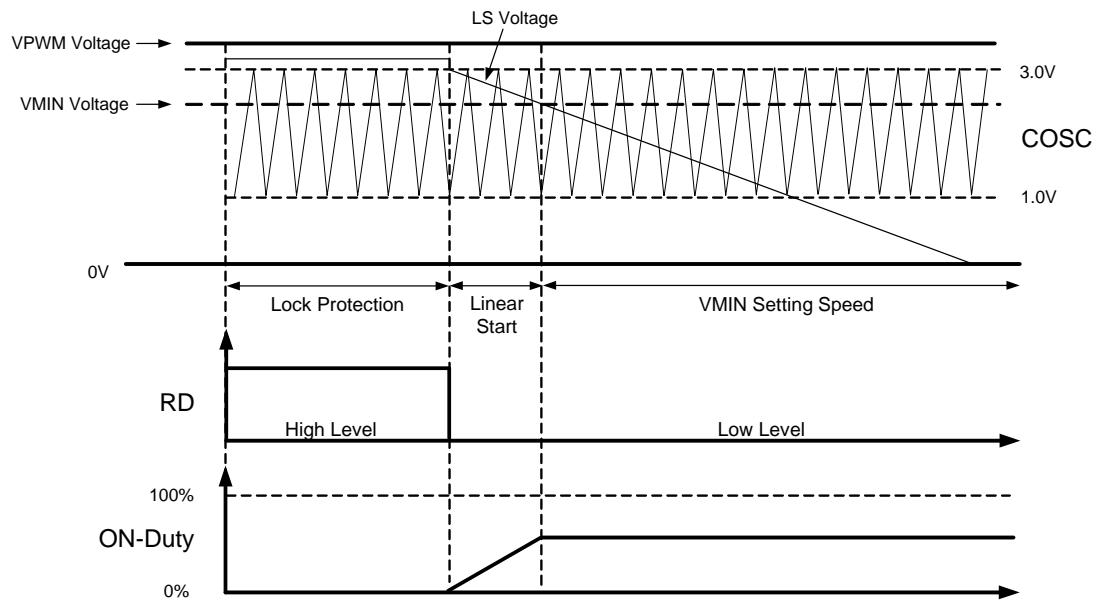
Figure 12. Operating Diagram 4 of AM4967 (Note 4)
