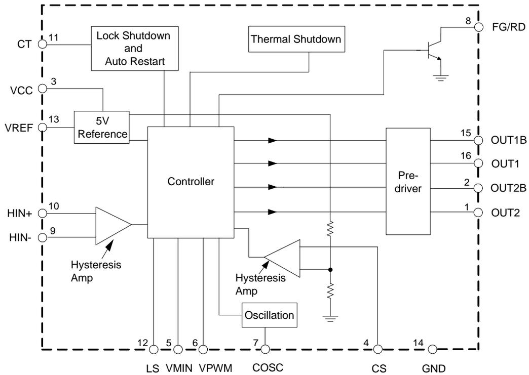
Figure 3. Functional Block Diagram of AM4967
