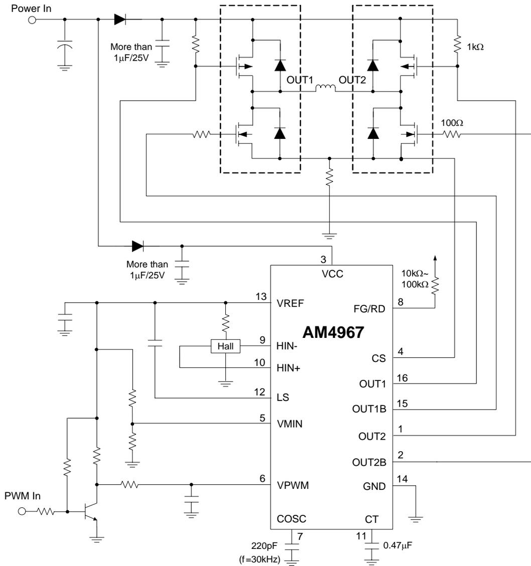
Figure 13. Typical Application of AM4967 ( $V_{CC}=12V$ )
