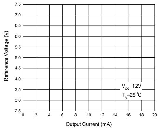
Figure 7. Reference Voltage vs. Output Current
