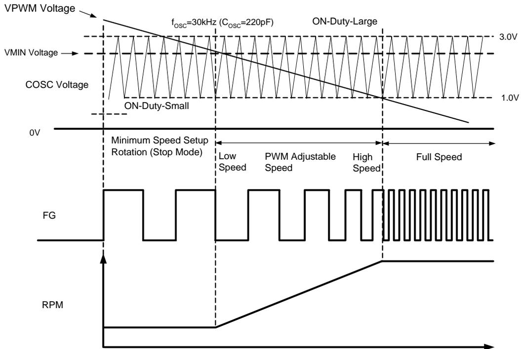
Figure 9. Operating Diagram 1 of AM4967 (Speed Control, Note 3)
