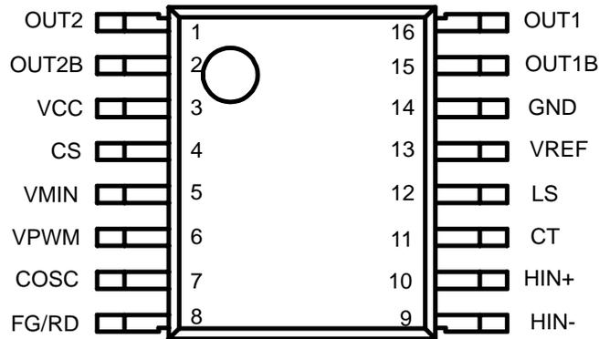
Figure 2. Pin Configuration of AM4967
