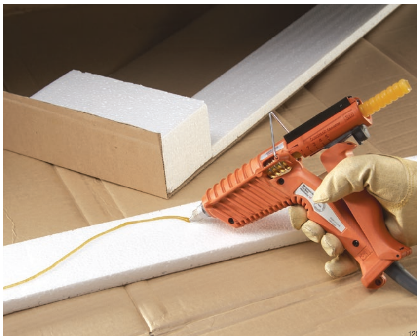
3M™ Hot Melt Applicator LT with 3M™ Hot Melt Adhesive 3762LM low temperature (265°F/129°C) adhesive effectively bonds heat-sensitive substrates such as styrene foam to itself, corrugated or other surfaces without damaging the foam.
