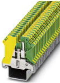
Ground modular terminal block, Connection method: Screw connection, Cross section: 0.2 mm 2 - 6 mm 2 , AWG 24 - 10, Width: 6.2 mm, Color: green-yellow, Mounting type: NS 35/15-2,3
