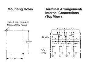
Note: Do not reverse the coil polarity.
