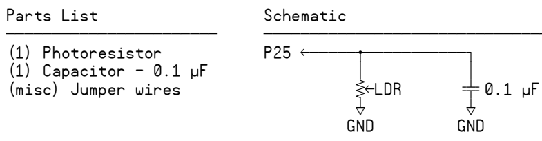
Figure 7-6: Second RC Decay Parts and Circuit
