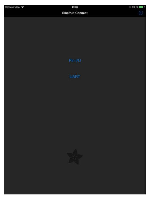
This will establish a connection between the nRF8001 and your iOS device, and you should see an I/O screen that allows you to select any available pin.
