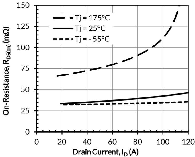
Figure 5. Typical drain-source on-resistances at  $V_{GS} = 12\text{V}$
