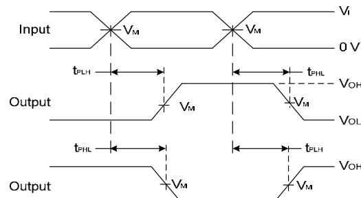
Voltage Waveform Propagation Delay Times
