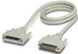
Assembled D-SUB cable shielded, 25-pos., stranded (7-wire), cable color RAL 7000 (gray), IP20 degree of protection, head 1 with socket shell 3 and straight cable outlet, head 2 with pin shell 3 and straight cable outlet, length: 1 m
