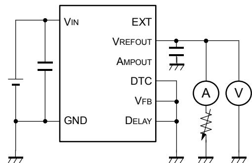
**Fig.10 V<sub>REFOUT</sub> Voltage Test Current**
