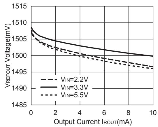
**25) V<sub>REFOUT</sub> Voltage vs. Output Current (2) (T<sub>opt</sub>=25°C) 26) Error Amplifier Gain/Phase vs. Frequency (T<sub>opt</sub>=25°C)
