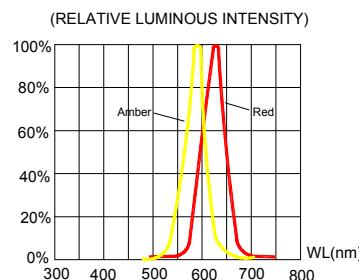
FIG.4 RELATIVE LUMINOUS INTENSITY VS.
