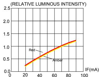
FIG.2 RELATIVE LUMINOUS INTENSITY VS.
