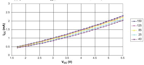
Figure 4-121. Idle Supply Current versus  $5V_{CC}$  (Internal RC Oscillator, 128kHz)
