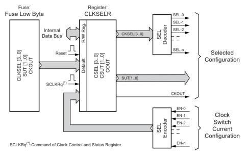
The CLKSELR register contains the CSEL, CSUT and COUT values which will be used by the 'Enable/Disable Clock Source', 'Request for Clock Availability' or 'Clock Source Switching' commands.
