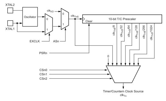
The clock source for Timer/Counter0 is named  $clk_{TOS}$ .  $clk_{TOS}$  is by default connected to the main system I/O clock  $clk_{IO}$ . By setting the AS0 bit in ASSR, Timer/Counter0 is asynchronously clocked from the XTAL oscillator or XTAL1 pin. This enables use of Timer/Counter0 as a real time counter (RTC).
