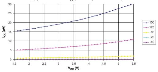
Figure 4-123. Power-down Supply Current versus V<sub>CC</sub> (Watchdog Timer Enabled)
