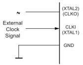
When this clock source is selected, start-up times are determined by the SUT Fuses or CSUT field as shown in Table 4-13 This external clock can be used by the asynchronous timer if the high or low frequency Crystal Oscillator is not running (see Section 4.5.3.3 "Enable/Disable Clock Source" on page 54). The asynchronous timer is then able to enable this input.
