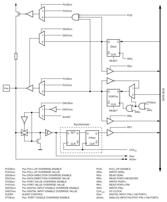
Note: 1. WRx, WPx, WDx, RRx, RPx, and RDx are common to all pins within the same port. clk<sub>I/O</sub>, SLEEP, and PUD are common to all ports. All other signals are unique for each pin.
