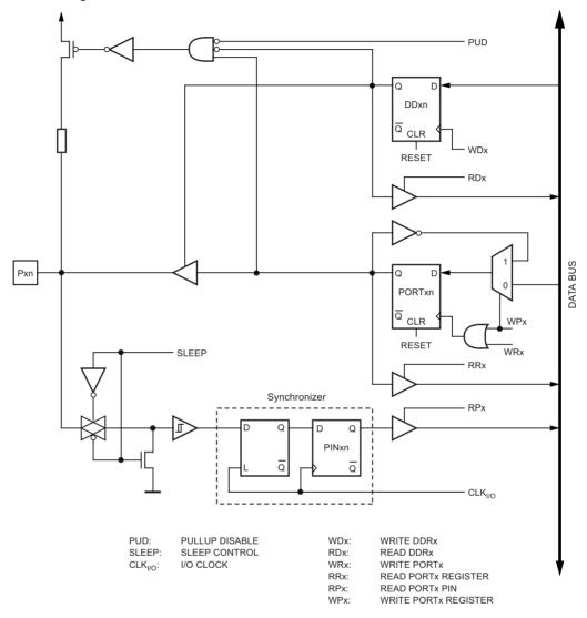
Note: 1. WRx, WPx, WDx, RRx, RPx, and RDx are common to all pins within the same port. clk<sub>I/O</sub>, SLEEP, and PUD are common to all ports.
