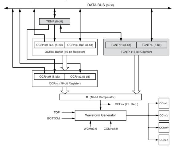
The OCR1A/B register is double buffered when using any of the twelve pulse width modulation (PWM) modes. For the normal and clear timer on compare (CTC) modes of operation, the double buffering is disabled. The double buffering synchronizes the update of the OCR1A/B compare register to either TOP or BOTTOM of the counting sequence. The synchronization prevents the occurrence of odd-length, non-symmetrical PWM pulses, thereby making the output glitch-free.
