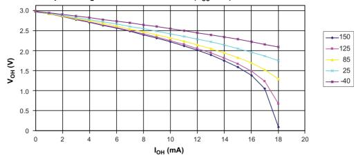
Figure 4-131. I/O Pin Output Voltage versus Source Current ( $V_{CC} = 5V$ )
