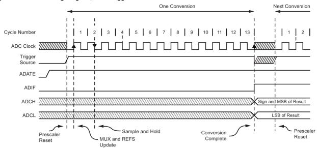
Figure 4-88. ADC Timing Diagram, Free Running Conversion
