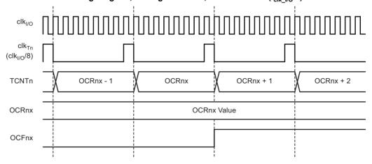
Figure 4-40 shows the setting of OCF0A and the clearing of TCNT0 in CTC mode.
