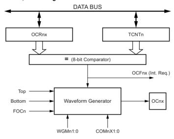
The OCR0A register is double buffered when using any of the pulse width modulation (PWM) modes. For the normal and clear timer on compare (CTC) modes of operation, the double buffering is disabled. The double buffering synchronizes the update of the OCR0A compare register to either top or bottom of the counting sequence. The synchronization prevents the occurrence of odd-length, non-symmetrical PWM pulses, thereby making the output glitch-free.
