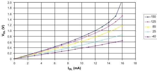
Figure 4-129. I/O Pin Output Voltage versus Sink Current (V<sub>CC</sub> = 5V)
