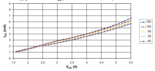
Figure 4-118. Active Supply Current versus V<sub>CC</sub> (Internal RC Oscillator, 128kHz)
