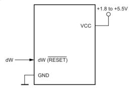
Figure 4-95 shows the schematic of a target MCU, with debugWIRE enabled, and the emulator connector. The system clock is not affected by debugWIRE and will always be the clock source selected by the CKSEL fuses.
