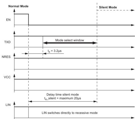
Figure 3-3. Switch to Silent Mode
