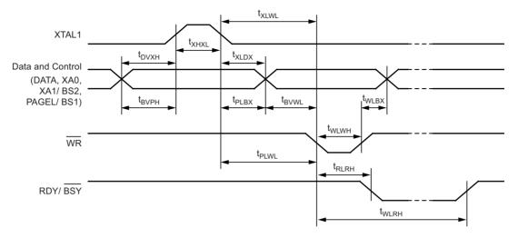
Figure 4-110. Parallel Programming Timing, Loading Sequence with Timing Requirements<sup>(1)</sup>
