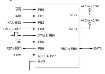
Note:  $V_{CC} - 0.3V < AV_{CC} < V_{CC} + 0.3V$ , however,  $AV_{CC}$  should always be within 4.5 to 5.5V
