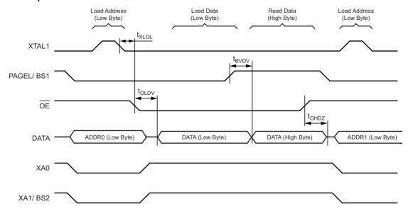
Note: 1. The timing requirements shown in Figure 4-109 (i.e.,  $t_{DVXH}$ ,  $t_{XHXL}$ , and  $t_{XLDX}$ ) also apply to reading operation.
