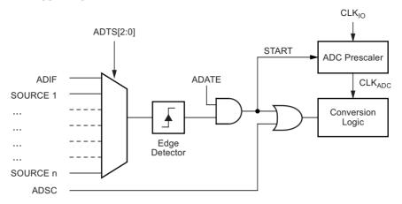
Using the ADC interrupt flag as a trigger source makes the ADC start a new conversion as soon as the ongoing conversion has finished. The ADC then operates in free running mode, constantly sampling and updating the ADC data register. The first conversion must be started by writing a logical one to the ADSC bit in ADCSRA register. In this mode the ADC will perform successive conversions independently of whether the ADC interrupt flag, ADIF is cleared or not.
