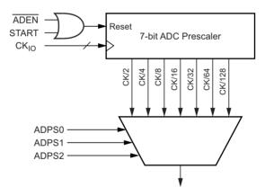
By default, the successive approximation circuitry requires an input clock frequency between 50kHz and 200kHz to get maximum resolution. If a lower resolution than 10bits is needed, the input clock frequency to the ADC can be higher than 200kHz to get a higher sample rate.
