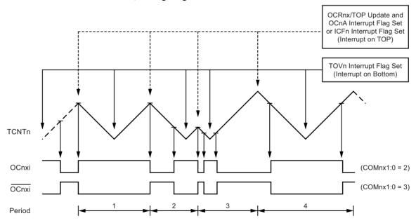
The Timer/Counter overflow Flag (TOV1) is set each time the counter reaches BOTTOM. When either OCR1A or ICR1 is used for defining the TOP value, the OC1A or ICF1 flag is set accordingly at the same timer clock cycle as the OCR1A/B Registers are updated with the double buffer value (at TOP). The interrupt flags can be used to generate an interrupt each time the counter reaches the TOP or BOTTOM value.
