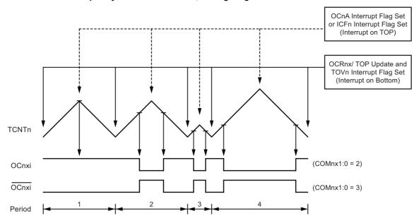
The Timer/Counter overflow flag (TOV1) is set at the same timer clock cycle as the OCR1A/B registers are updated with the double buffer value (at BOTTOM). When either OCR1A or ICR1 is used for defining the TOP value, the OC1A or ICF1 flag set when TCNT1 has reached TOP. The interrupt flags can then be used to generate an interrupt each time the counter reaches the TOP or BOTTOM value.
