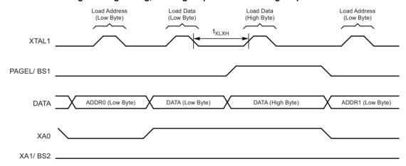
Note: 1. The timing requirements shown in Figure 4-109 (i.e.,  $t_{DVXH}$ ,  $t_{XHXL}$ , and  $t_{XLDX}$ ) also apply to loading operation.
