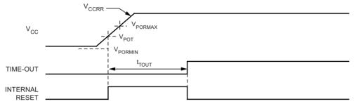
Figure 4-18. MCU Start-up, RESET Extended Externally
