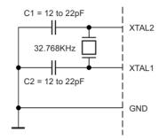
12 to 22pF capacitors may be necessary if parasitic impedance (pads, wires and PCB) is very low.
