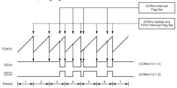
The Timer/Counter overflow flag (TOV0) is set each time the counter reaches MAX. If the interrupt is enabled, the interrupt handler routine can be used for updating the compare value.
