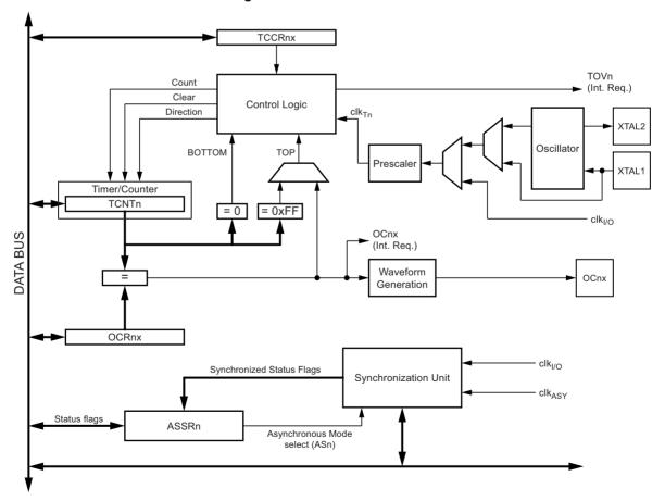
The Timer/Counter (TCNT0) and output compare register (OCR0A) are 8-bit registers. Interrupt request (shorten as Int.Req.) signals are all visible in the timer interrupt flag register (TIFR0). All interrupts are individually masked with the timer interrupt mask register (TIMSK0). TIFR0 and TIMSK0 are not shown in the figure.
