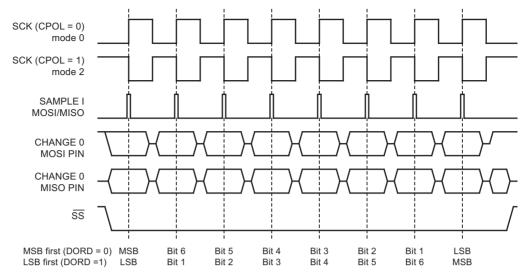
Figure 4-61. SPI Transfer Format with CPHA = 1
