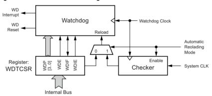
The 'Enable Watchdog in Automatic Reload Mode' command has priority over the standard watchdog enabling. In this mode, only the reset function of the watchdog is enabled (no more watchdog interrupt). The WDP3..0 bits of the WDTCSR register always determine the watchdog timer prescaling.
