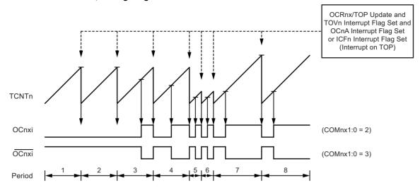
The Timer/Counter overflow flag (TOV1) is set each time the counter reaches TOP. In addition the OC1A or ICF1 flag is set at the same timer clock cycle as TOV1 is set when either OCR1A or ICR1 is used for defining the TOP value. If one of the interrupts are enabled, the interrupt handler routine can be used for updating the TOP and compare values.
