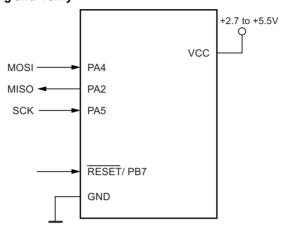
Note: 1. If the device is clocked by the internal oscillator, it is no need to connect a clock source to the XTAL1 pin.
