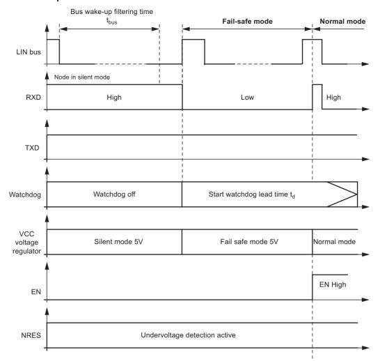
Figure 3-4. LIN Wake-up from Silent Mode
