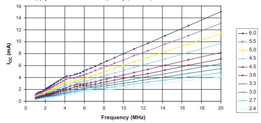
Figure 4-117. Active Supply Current versus V<sub>CC</sub> (Internal RC Oscillator, 8MHz)
