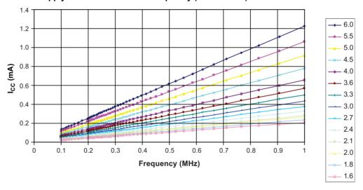
Figure 4-116. Active Supply Current versus Frequency (≥ 1MHz)
