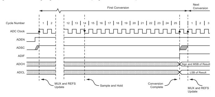
Figure 4-86. ADC Timing Diagram, Single Conversion
