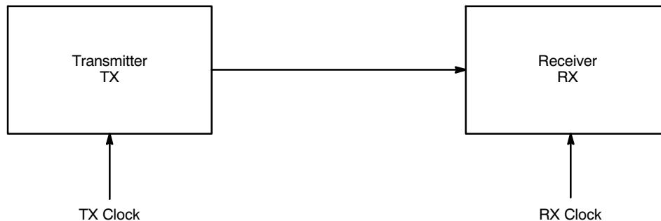
Figure 33. Example of a Serial Data Transmission System
