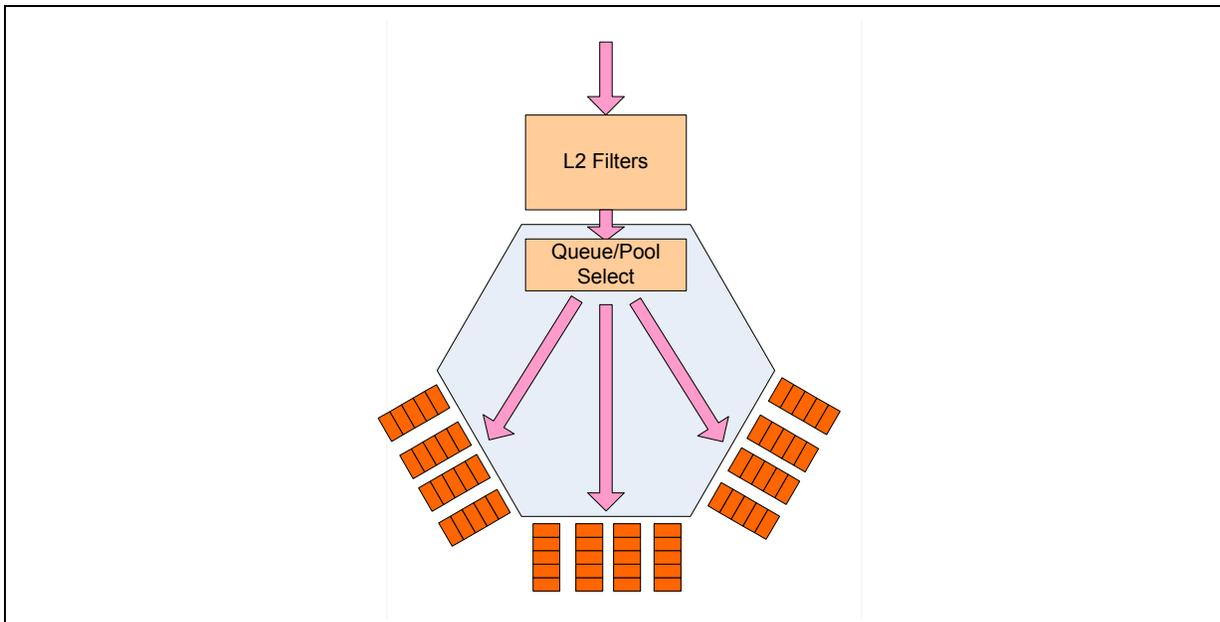
In the third stage, a received packet that successfully passed the Rx filters is associated with one or more receive descriptor queues as described in this section.
