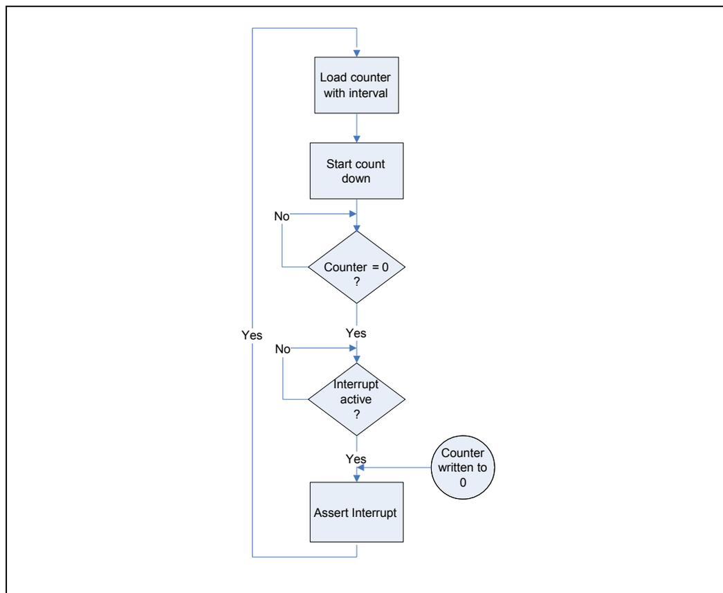
For cases where the Controller is connected to a small number of clients, it is desirable to fire off the interrupt as soon as possible with minimum latency. For these cases, when the EITR counter counts down to zero and no interrupt event has happened, then the EITR counter is not re-armed but stays at zero. Thus, the next interrupt event triggers an interrupt immediately. That scenario is illustrated as "Case B" below.
