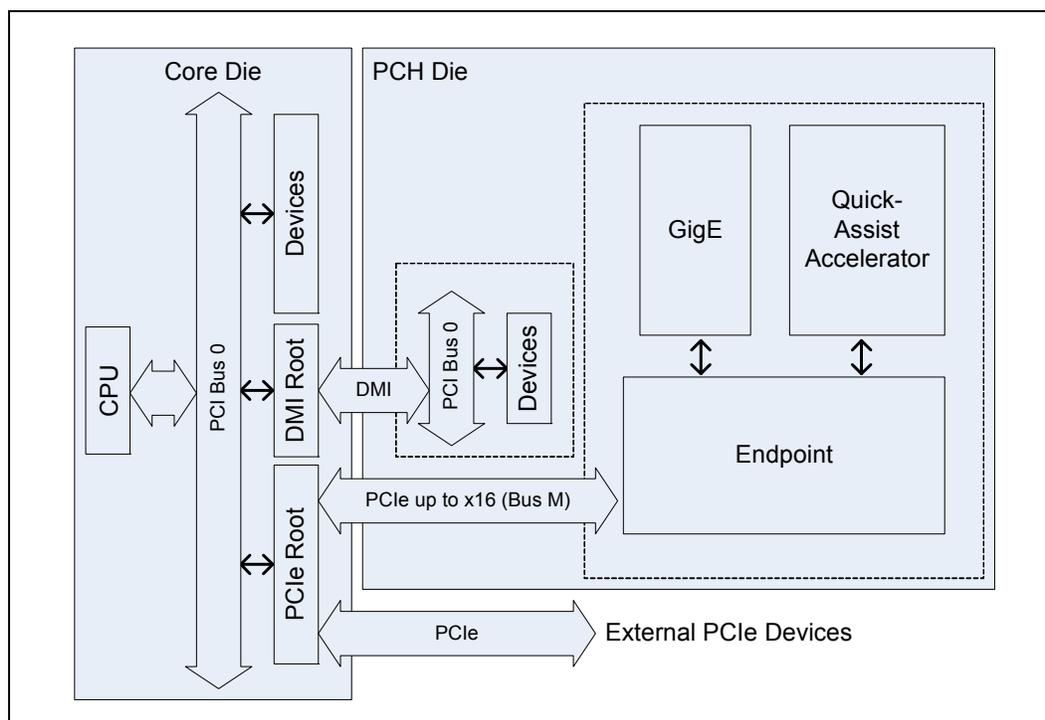
In the figure above, PCI bus 0 originates in the CPU die and reaches internal PCI devices through internal paths. Bus 0 is bridged into the PCH via an DMI interconnect and into the PCIe\* Endpoint via a subset of the PCI Express lanes on the CPU die. The PCIe Express Endpoint materializes the individual functions of the endpoint device on bus M as the figure illustrates.
