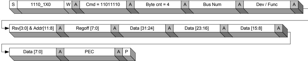
**Figure 4-12. SMBus Block-Size Memory Register Write**
