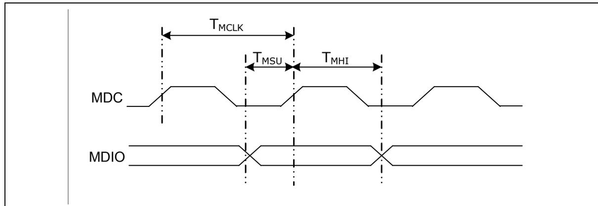
**Figure 33-18. MDIO Output AC Timing Diagram**
