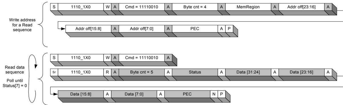
**Figure 4-7. SMBus Word-Size Configuration Register Read**
