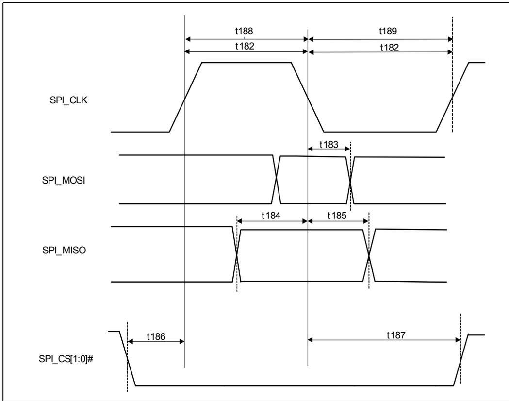
**Note:** t184 and t185 are referencing clock edge where the PCH will sample the SPI\_MISO pin. The slave transmitted this bit on the previous falling clock edge which is not shown.
