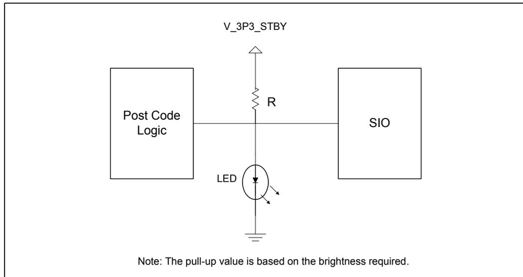
The anticipated usage model is that either the system or the SIO can drive a pin low to turn off an LED. In the case of the power LED, the SIO would normally leave its corresponding pin in a high-Z state to allow the LED to turn on. In this state, the system can blink the LED by driving its corresponding pin low and subsequently tri-stating the buffer. The I/O buffer should not drive a '1' when configured for this functionality and should be capable of sinking 24mA of current.
