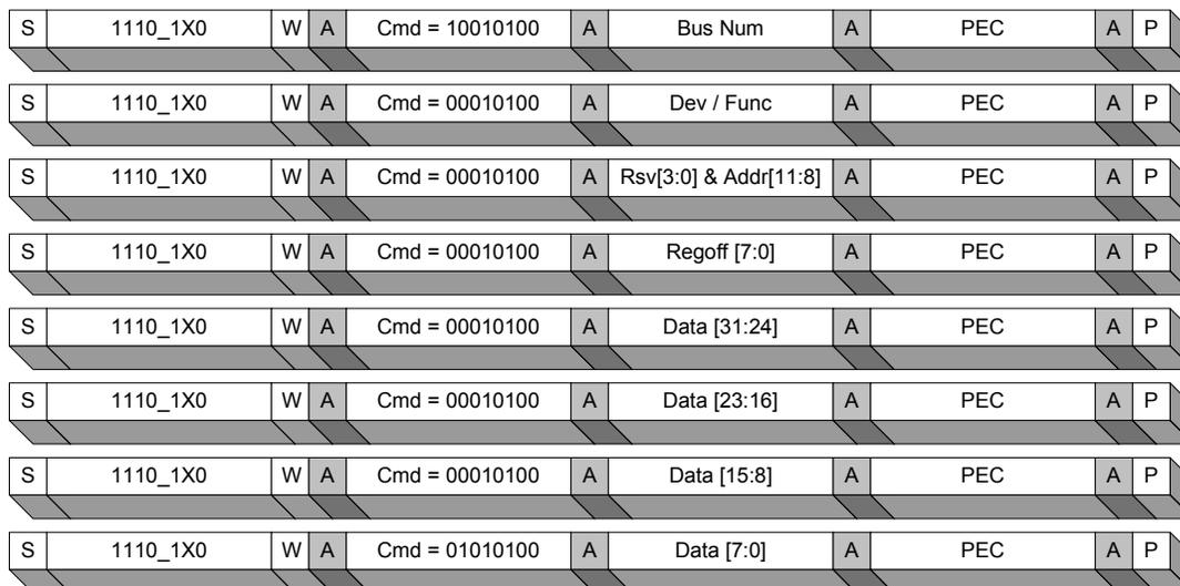
**Figure 4-16. SMBus Memory (Byte Write, PEC Enabled)**
