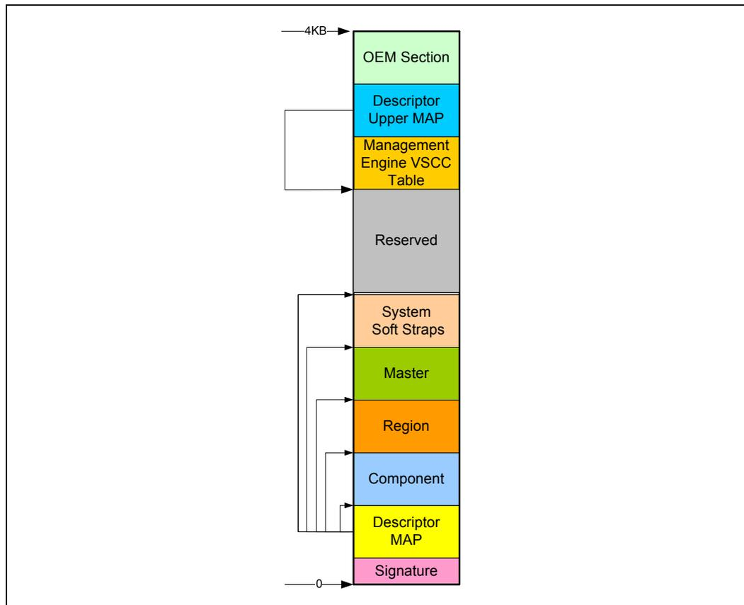
1. The Flash Signature selects Descriptor Mode and verifies if the flash is programmed and functioning. The data at the bottom of the flash (offset 0) must be 0FF0A55Ah to be in Descriptor mode.
