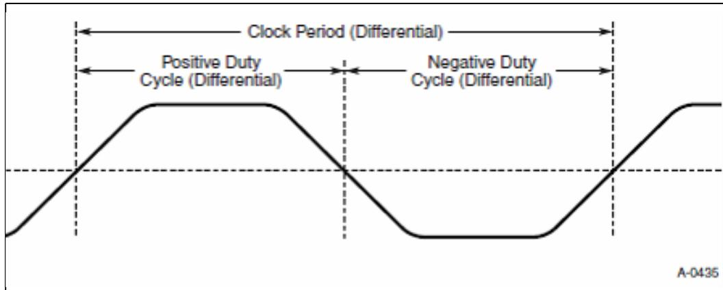
Figure 33-12. Differential Measurement Point for Rise and Fall Time
