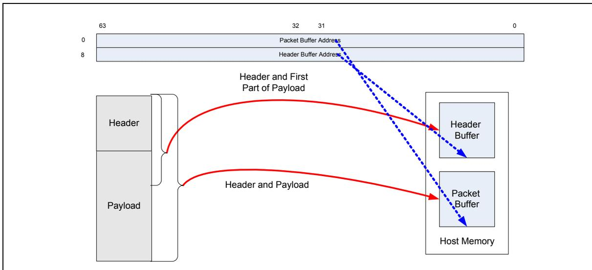
The physical address of each buffer is written in the *Buffer Addresses* fields. The sizes of these buffers are statically defined by *BSIZEPACKET* and *BSIZEHEADER* fields in the *SRRCTL[n]* registers.
