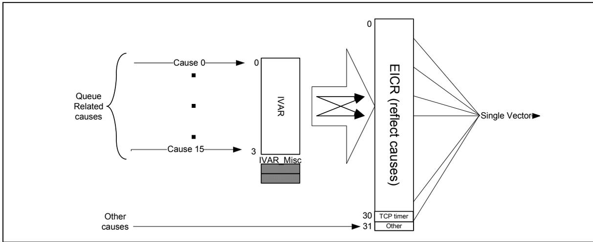
The table below maps the different interrupt causes into the IVAR registers.
