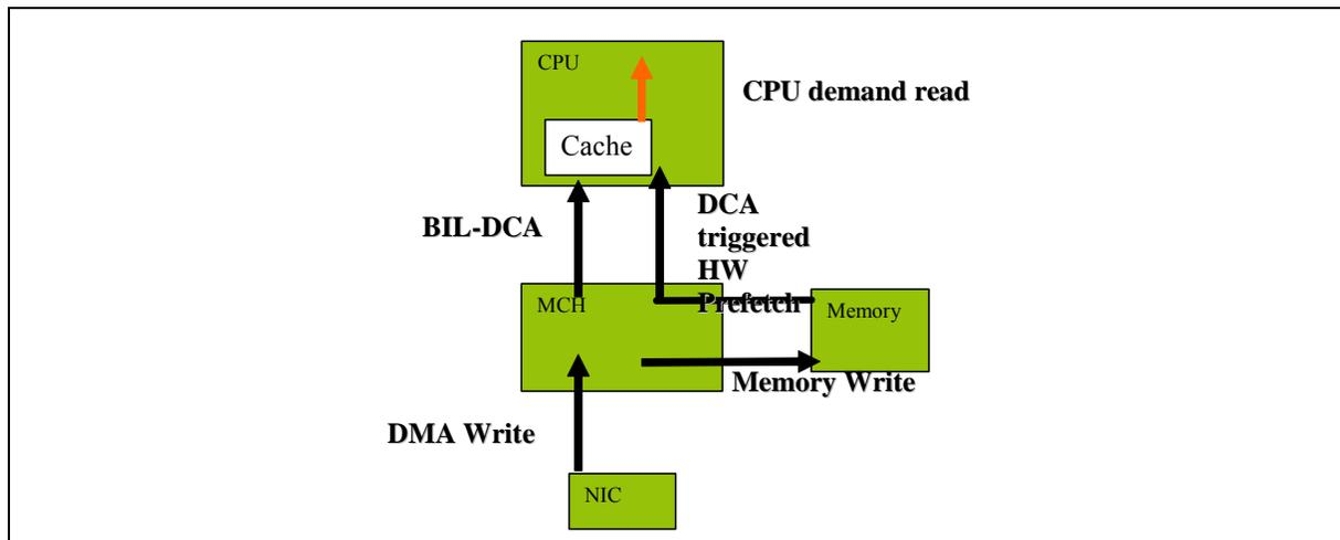
As shown in [Figure 26-26](#), DCA provides a mechanism where the posted write data from an I/O device, such as an Ethernet NIC, can be placed into CPU cache with a hardware pre-fetch. This mechanism is initialized upon a power good reset. A software device driver for the I/O device configures the I/O device for DCA and sets up the appropriate DCA target ID for the device to send data.
