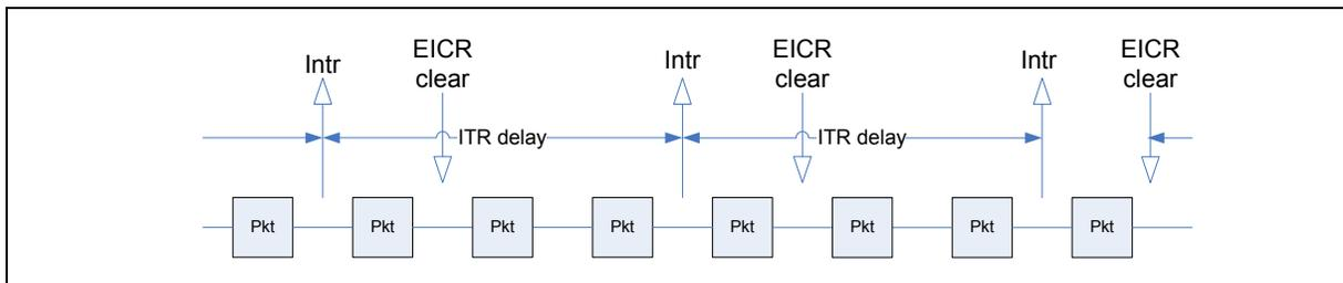
**Figure 26-24. Light Load, Interrupts Immediately on Packet Receive**
