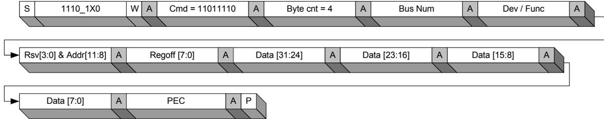
**Figure 4-12. SMBus Block-Size Memory Register Write**
