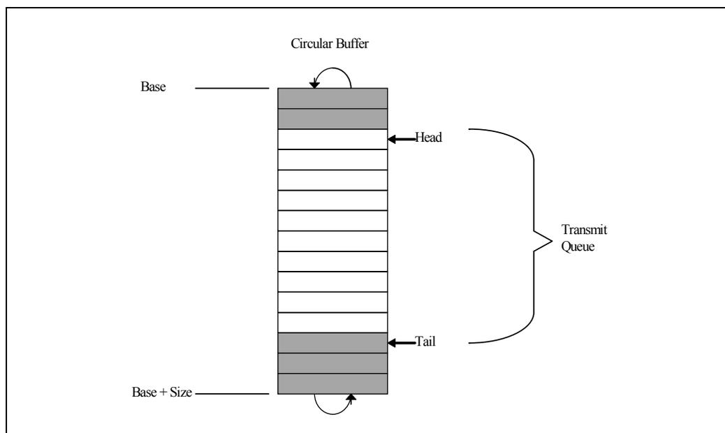
The shaded boxes in the figure represent descriptors that are not currently owned by hardware that software can modify.
