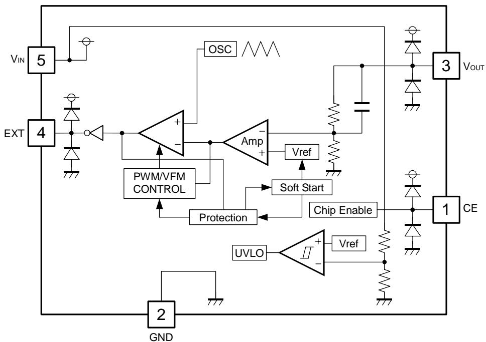
**\*Adjustable Output Voltage Type**
