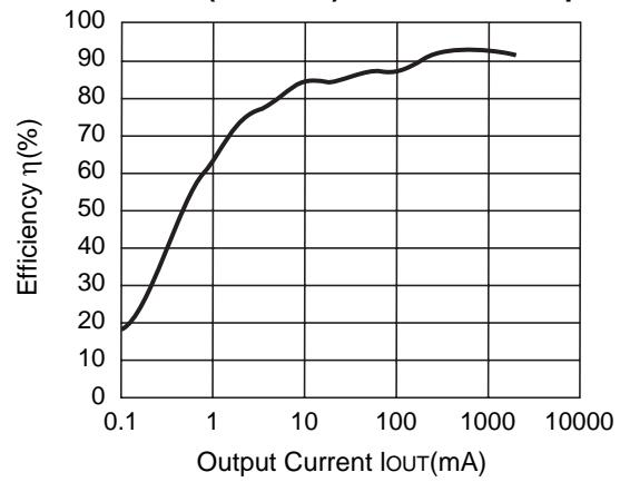
R1224N332L ( $V_{IN}=4.8V$ ) CDRH127-27 $\mu$ H
