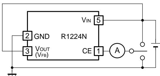
**Output Delay Time for Protection Circuit**
