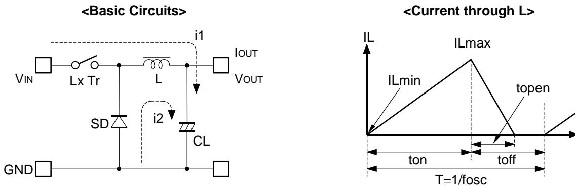
Step 1:  $Lx\ Tr.$  turns on and current  $IL$  ( $=i_1$ ) flows, and energy is charged into  $CL$ . At this moment,  $IL$  increases from  $IL_{min}$  ( $=0$ ) to reach  $IL_{max}$  in proportion to the on-time period ( $ton$ ) of  $Lx\ Tr.$
