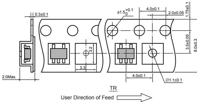
**TAPING REEL DIMENSIONS REUSE REEL (EIAJ-RRM-08Bc)**
