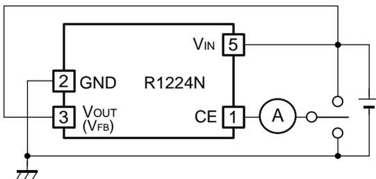
Output Delay Time for Protection Circuit
