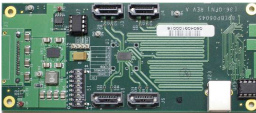
89KT0604S 2-lane, with I 2 C Configuration
