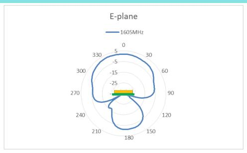
Glonass Radiation pattern on 70mmX70mm metal plane
