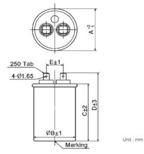
\$3 Other shape and specific requirement can be designed. Please contact, if necessary. Three tabs and as many as four tabs are also possible though standards of the number of terminal tabs are two tabs.
