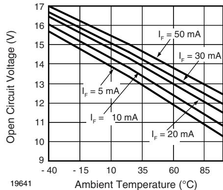
Fig. 5 - Open Circuit Voltage vs. Temperature
