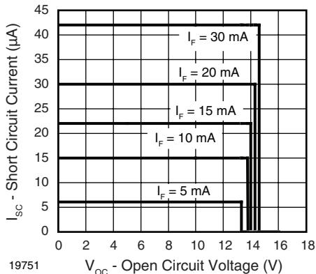
Fig. 1 - Short Circuit Current vs. Open Circuit Voltage
