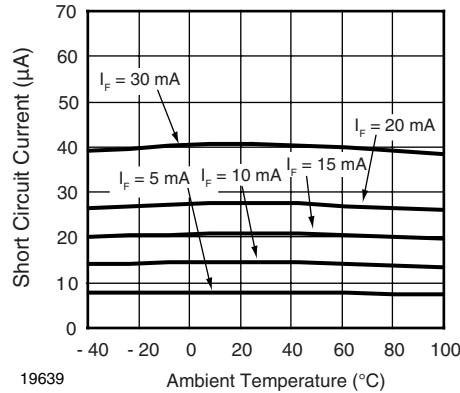
Fig. 4 - Short Circuit Current vs. Temperature
