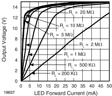
Fig. 2 - Output Voltage vs. LED Current
