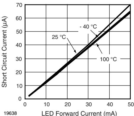
Fig. 3 -  $I_{sc}$  vs. LED Forward Current
