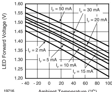
Fig. 6 - LED Forward Voltage vs. Temperature
