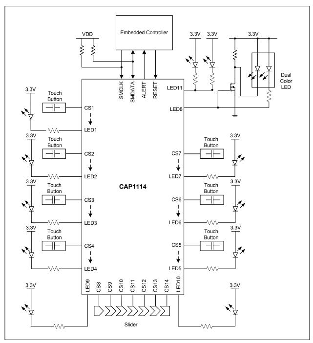
Figure 5.1 System Diagram for CAP1114
