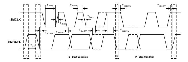
Figure 4.1 SMBus Timing Diagram
