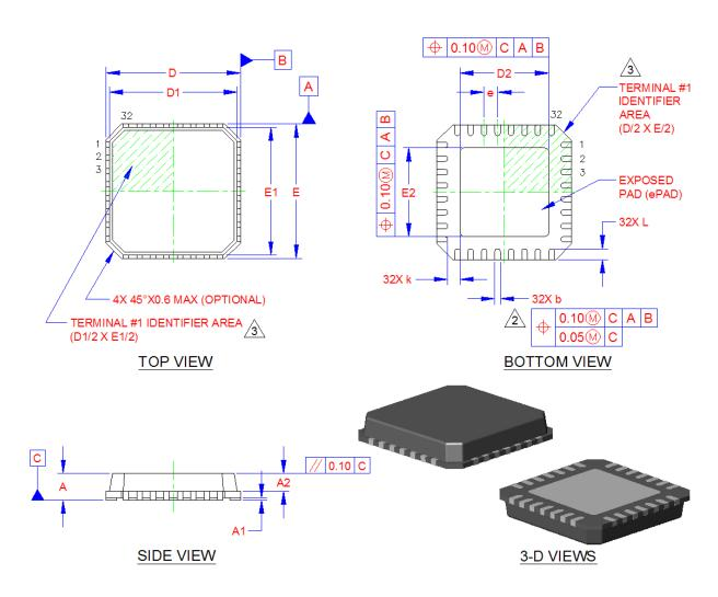
Figure 7.1 Package Diagram - 32-Pin QFN
