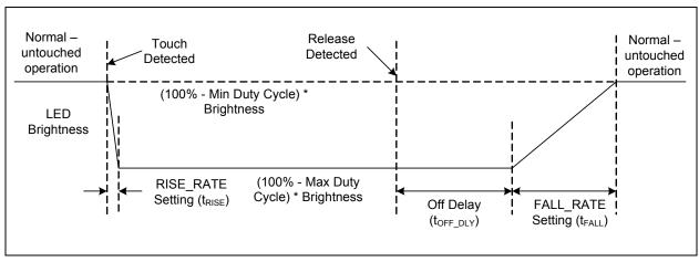
Figure 6.5 Direct Behavior for Non-Inverted Polarity
