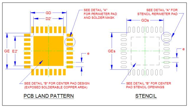
Figure 7.3 Package PCB Land Pattern and Stencil
