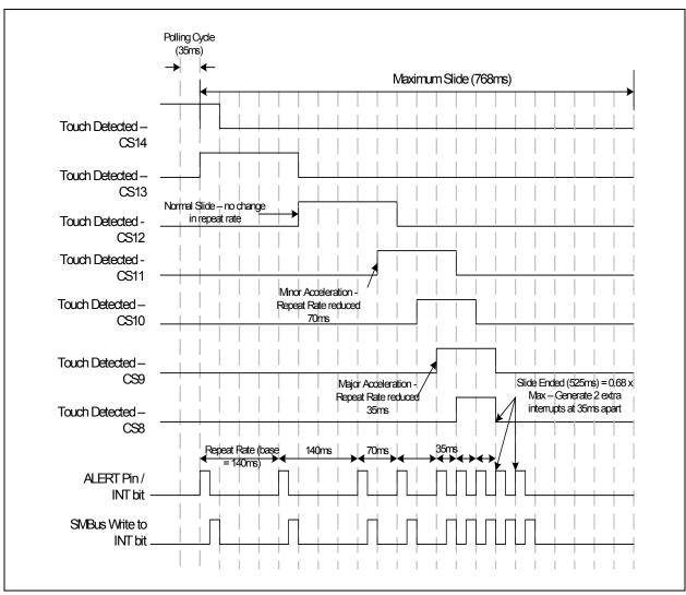
Figure 5.7 Slide Interrupt Behavior - Acceleration Example
