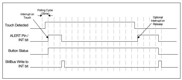
Figure 5.3 Button Interrupt Behavior - No Repeat Rate Enabled
