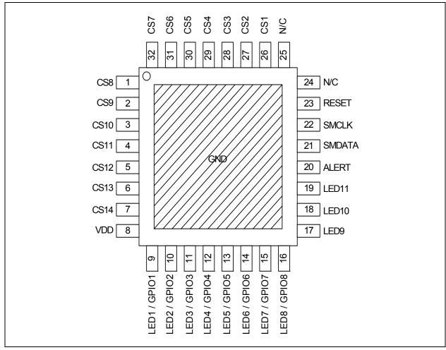
Figure 2.1 CAP1114 Pin Diagram (32-Pin QFN)
