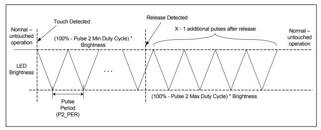
Figure 6.3 Pulse 2 Behavior with Non-Inverted Polarity
