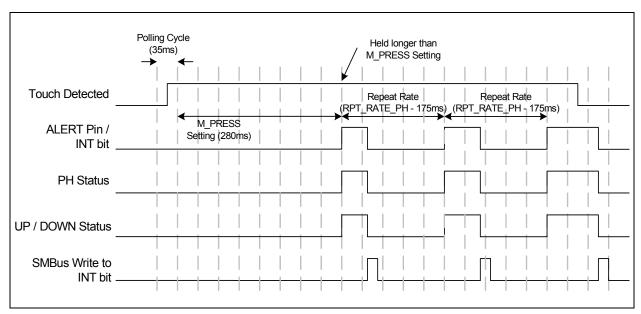
Figure 5.5 Press and Hold Interrupt Behavior
