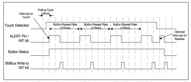
Figure 5.2 Button Interrupt Behavior - Repeat Rate Enabled (default)
