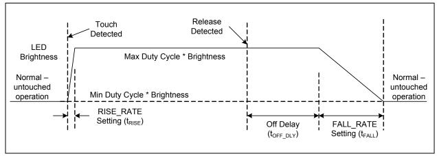
Figure 6.6 Direct Behavior for Inverted Polarity
