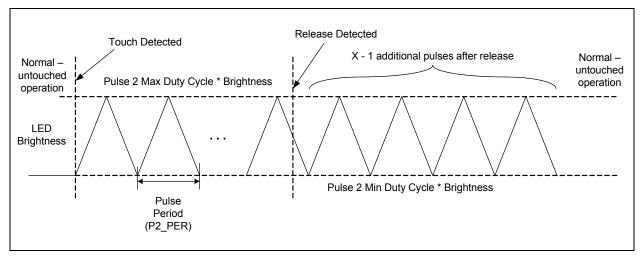
Figure 6.4 Pulse 2 Behavior with Inverted Polarity
