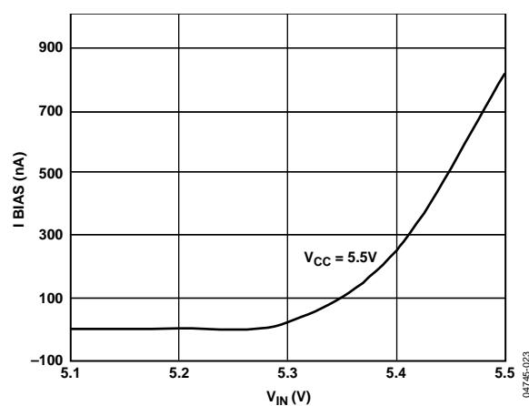
Figure 13. Input Bias Current vs. Input Voltage
