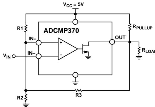
Figure 22. Inverting ADCMP370 Comparator Configuration with Hysteresis
