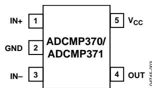
Figure 3. Pin Configuration
