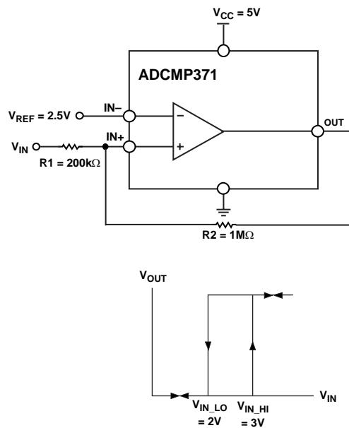
Figure 19. Noninverting ADCMP371 Comparator Configuration with Hysteresis
