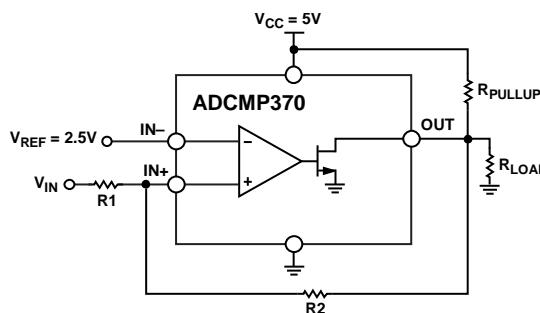
Figure 21. Noninverting ADCMP370 Comparator Configuration with Hysteresis
