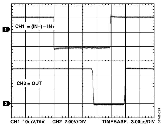
Figure 16. Propagation Delay Timing 10 mV Overdrive
