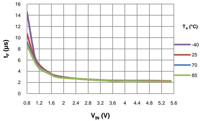
$t_{OFF}$  vs  $V_{IN}$ ,  $V_{BIAS}=2.5\text{V}$
