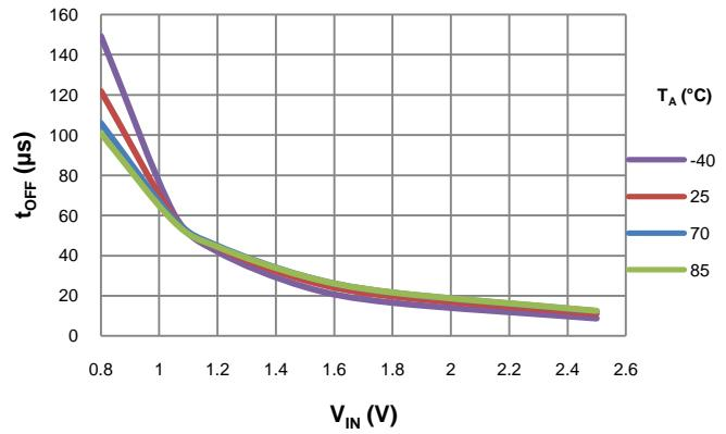
$t_{OFF}$  vs  $V_{IN}$ ,  $V_{BIAS}=5.5\text{V}$
