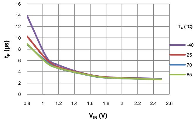
$t_F$  vs  $V_{IN}$ ,  $V_{BIAS}=5.5\text{V}$
