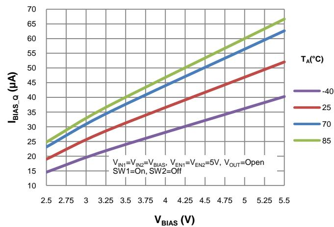
$V_{BIAS}$  vs. SHUTDOWN CURRENT (BOTH CHANNELS)
