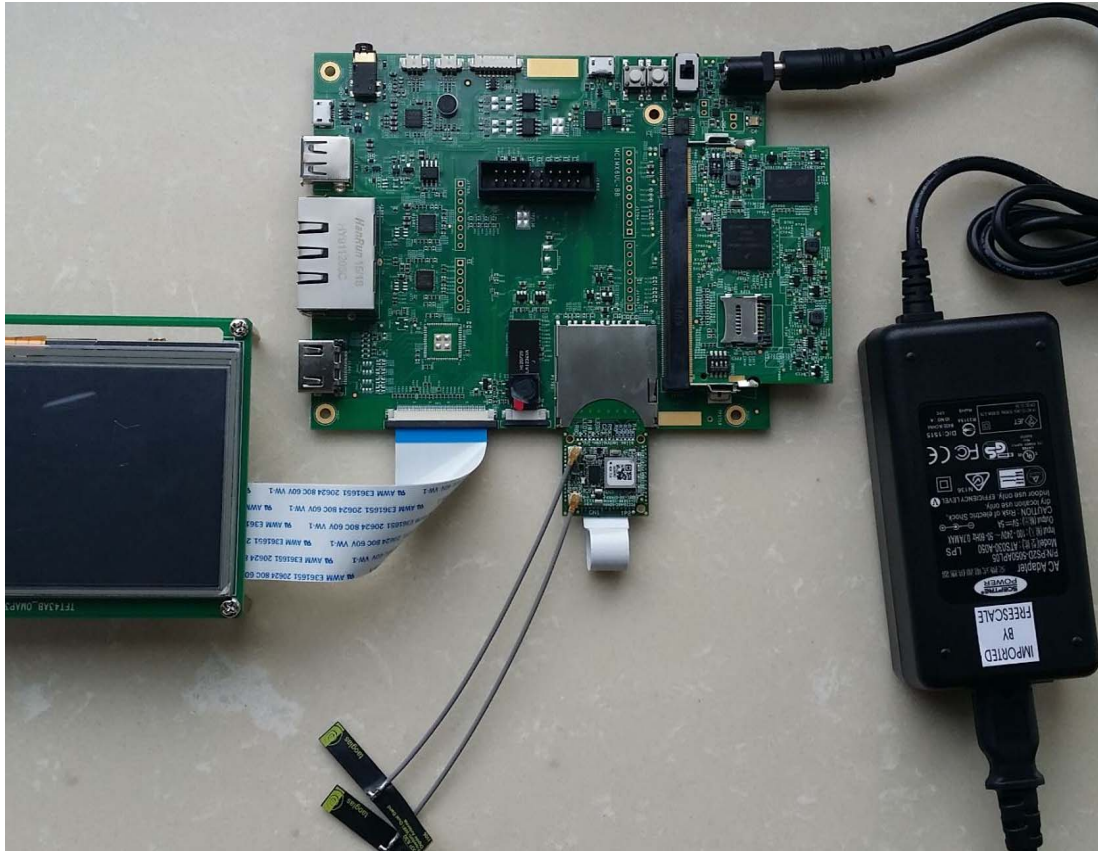
Figure 3. Overview of the i.MX 6UltraLite EVK board connection
