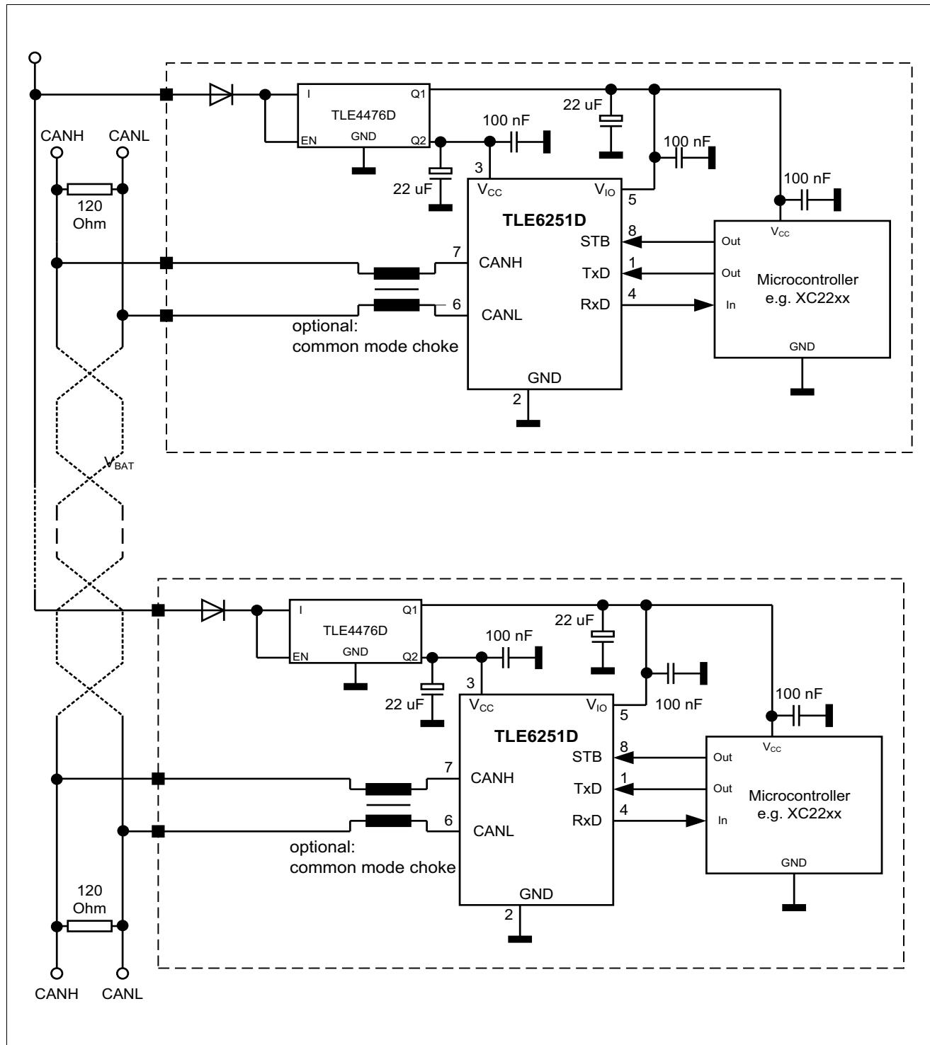
**Figure 11 Application circuit**
