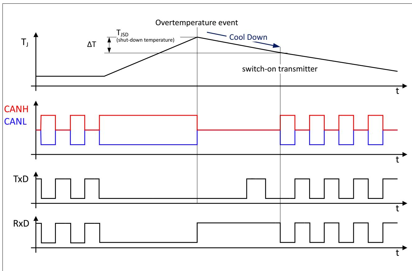
**Figure 8** Overtemperature protection
