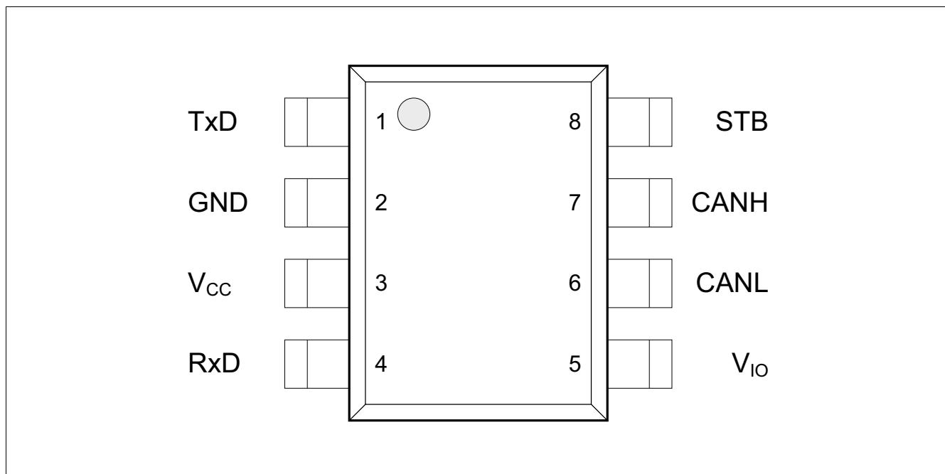
**Figure 2** Pin configuration
