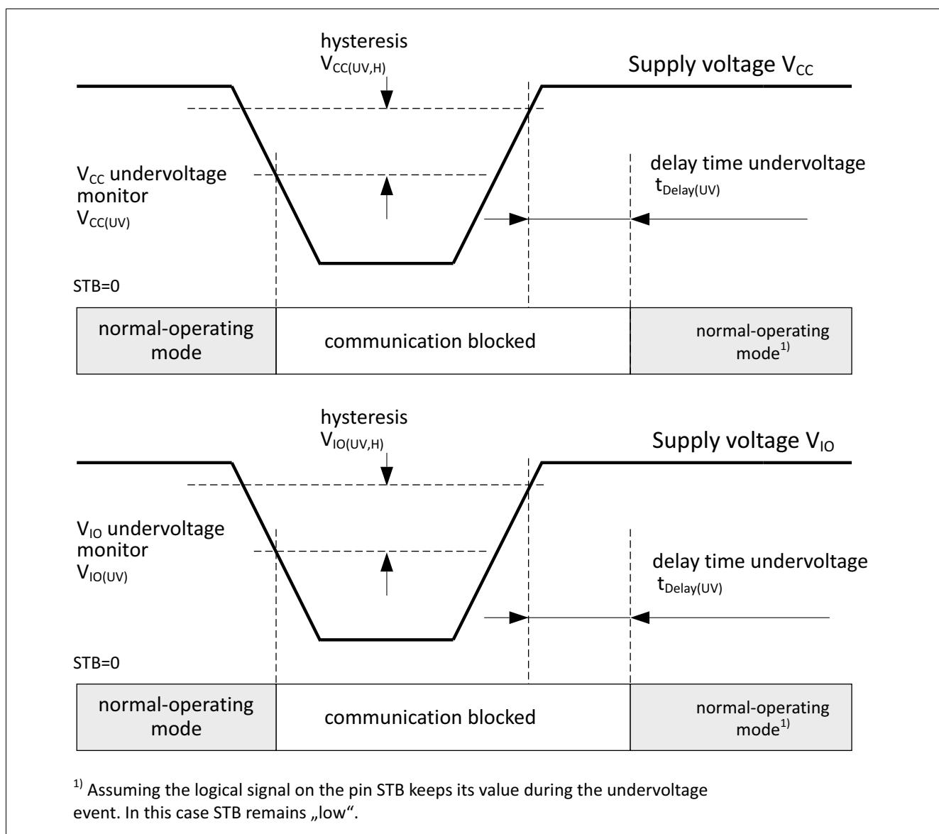
**Figure 7 Undervoltage detection on  $V_{CC}$  or  $V_{IO}$**
