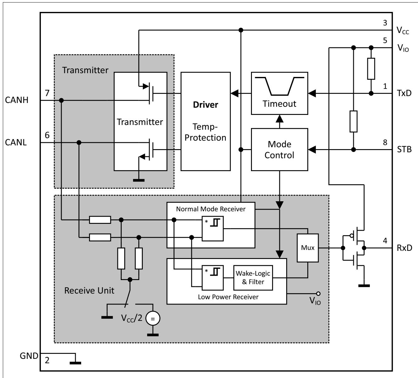
Figure 1 Block diagram
