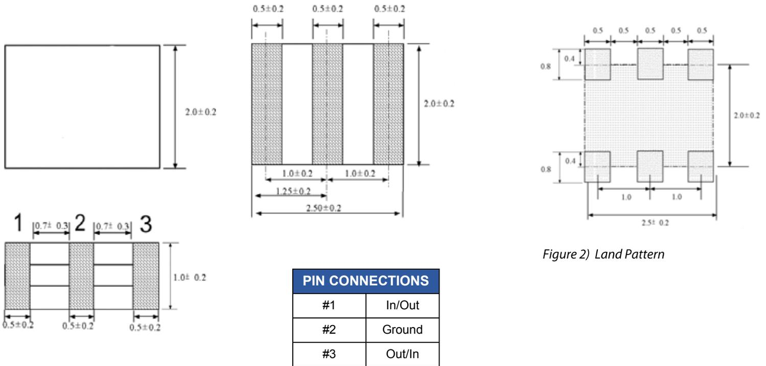
Figure 1) ECS-HFR-B Series - Top, Side and Bottom Views
