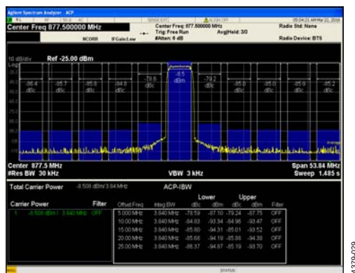
Figure 84. Single-Carrier W-CDMA at 877.5 MHz
