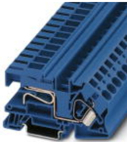
Installation level terminal block, Spring-cage connection, Cross section: 0.2 mm 2 - 16 mm 2 , AWG: 24 - 6, Width: 10 mm, Color: blue, Mounting type: NS 35/15, NS 35/7,5
