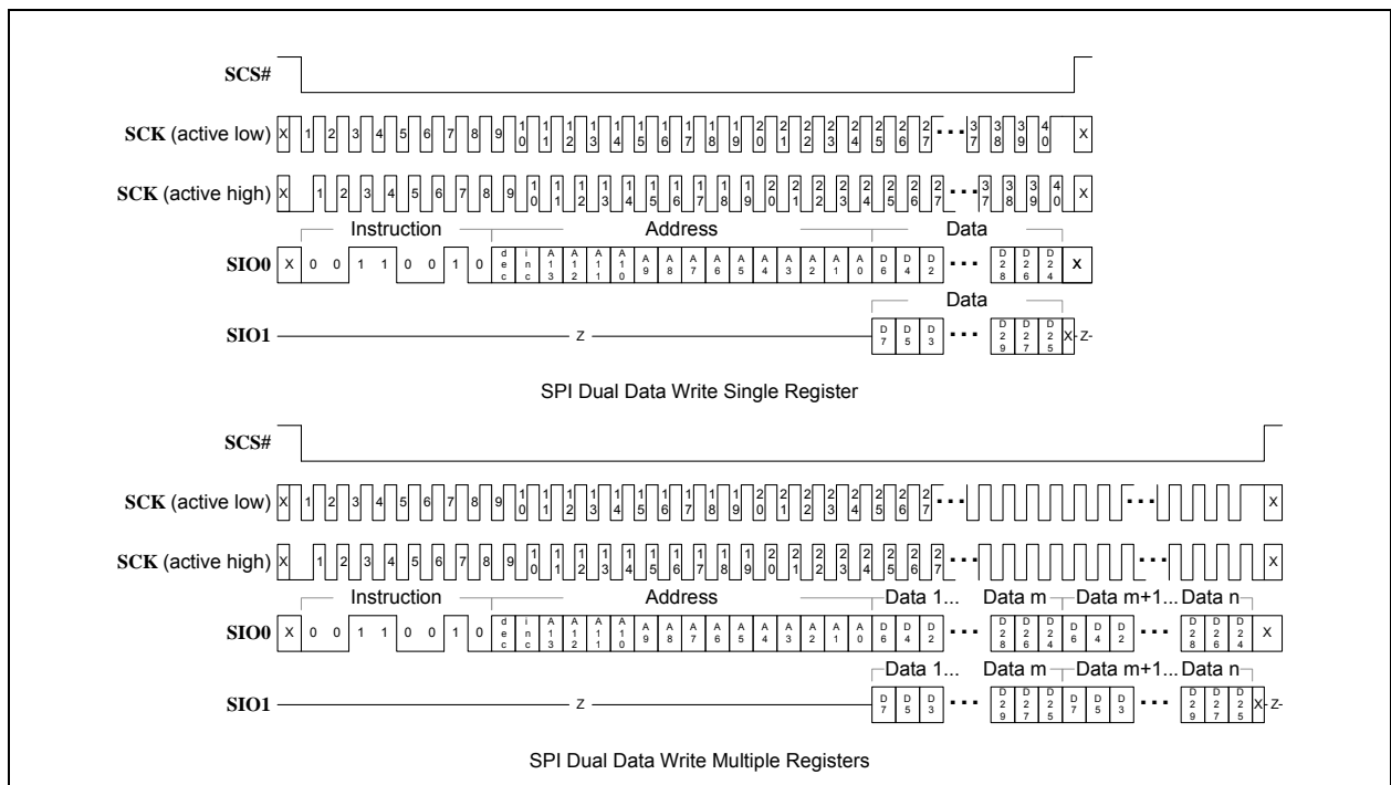
FIGURE 10-13: SPI DUAL DATA WRITE
