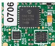
The MM7150 motion module consists of three chips: Bosch BMC150 accelerometer, Bosch BMG160 Gyroscope, and Microchip's SSC7150 motion coprocessor.
