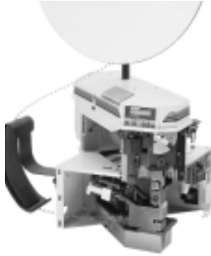
Model G Splice Terminating Machine, P/N 356462-2 & Applicator
