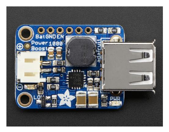
The PowerBoost 1000 has at the heart a TPS61030 boost converter from TI (https://adafru.it/dLY). This boost converter chip has some really nice extras such as low battery detection, 4A internal switch, synchronous conversion, excellent efficiency, and 700KHz high-frequency operation. Check out these specs!
