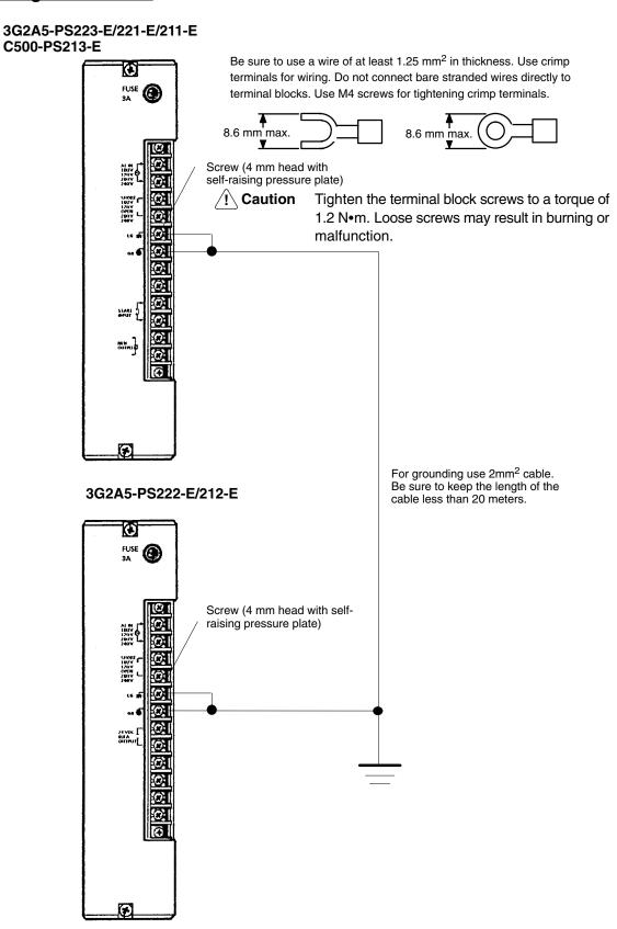
**Caution** Ground the Power Supplies separately from peripheral devices.
