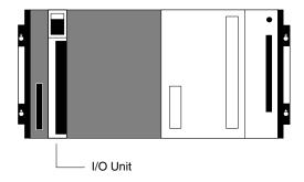
I/O Units are where the control connections are made from the PC to all the various input devices and output devices. As you can see from the figure, there is still some space available on the right side of the I/O Unit. This space is for any additional I/O Units that may be required.
