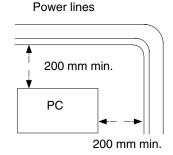
Whenever possible, use wiring conduit to hold the I/O wiring. Standard wiring conduit should be used, and it should be long enough to completely contain the I/O wiring and keep it separated from other cables.
