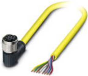
Sensor/Actuator cable, 8-position, PVC, yellow, Free cable end, on Socket angled M12-SPEEDCON, A-coded, Cable length: 2 m
