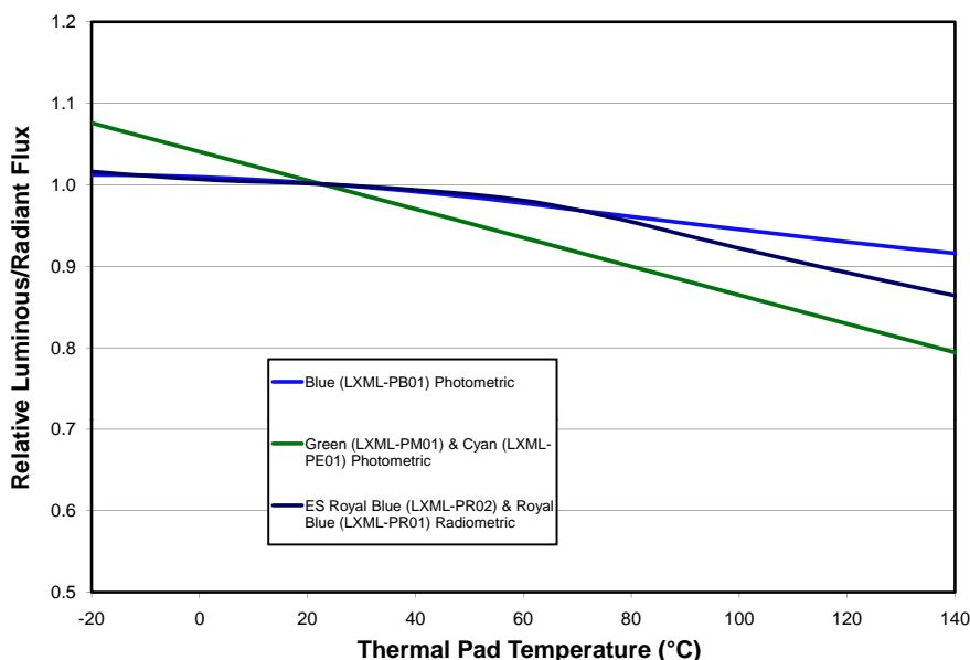
\*LXML-PR02 values are based on 700 mA drive current.
