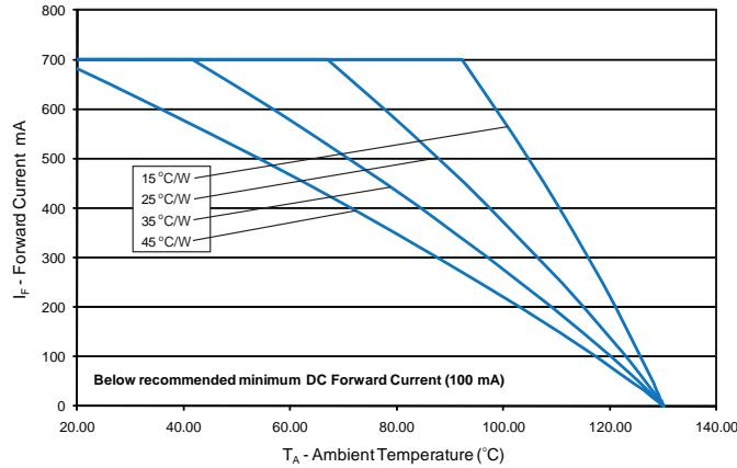
Figure 23. Maximum forward current vs. ambient temperature,
