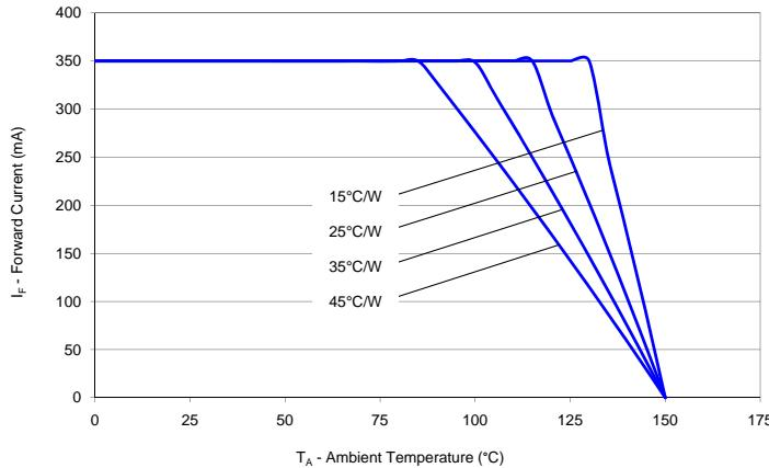
**Figure 15.** Maximum forward current vs. ambient temperature, based on  $T_{JMAX} = 150^\circ\text{C}$ , green LXML-PM01, cyan LXML-PE01, blue LXML-PB01 & royal-blue LXML-PR01 emitters.
