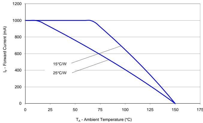
Figure 24. Maximum forward current vs. ambient temperature,
