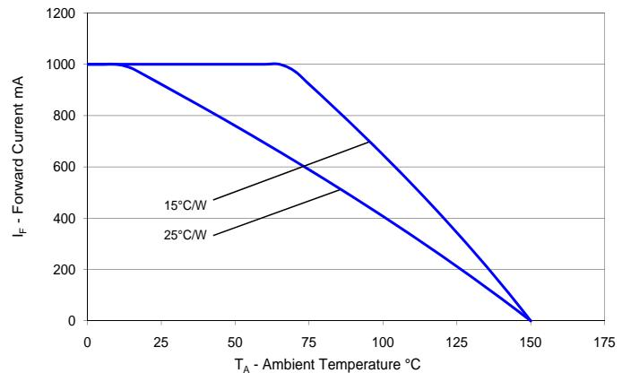
Figure 25. Maximum forward current vs. ambient temperature,
