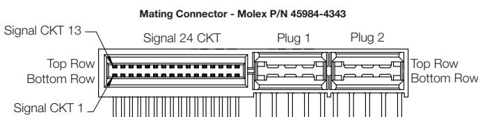
\*Note: The top side of the PSU Output Connector connects with the Bottom Row of the Mating Connector
