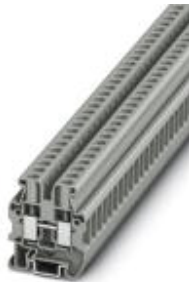
Mini feed-through terminal block, Connection method: Screw connection, Cross section: 0.2 mm 2 - 6 mm 2 , AWG: 24 - 10, Width: 6.2 mm, Color: gray, Mounting type: NS 15
