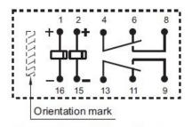
Diagram shows the "reset" position Energize terminals 1 and 16 to "set" Energize terminals 2 and 15 to "reset"
