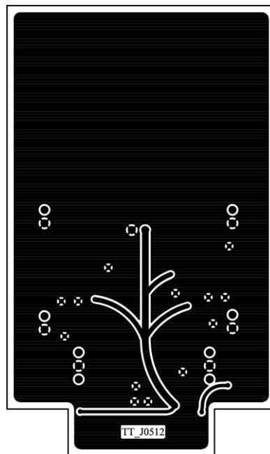
Figure 13. TS1004 Bottom Layer (GND) #1
