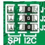
The Gyro Click™ board communicates with the main board microcontroller via I<sup>2</sup>C or SPI interface depending on the position of the **J1**, **J2** and **J3** SMD jumpers. These jumpers are soldered in I<sup>2</sup>C interface position by default. There is an option to select the alternate address with jumper **J4** in the case of I<sup>2</sup>C interface (default position is logic 1).
