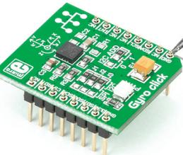
Turn the board upward again. Make sure to align the headers so that they are perpendicular to the board, then solder the pins carefully.
