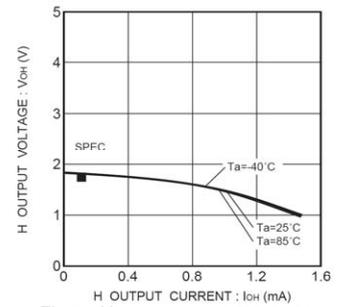
Fig.7 H output voltage  $V_{OH-IOH}$ ( $V_{CC}=1.8\text{V}$ )
