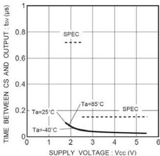
Fig.29 Time from CS to output establishment tSV
