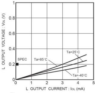
Fig.5 L output voltage  $V_{OL-IOL}$ ( $V_{CC}=2.5\text{V}$ )
