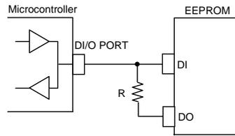
Fig.80 DI, DO control line common connection
