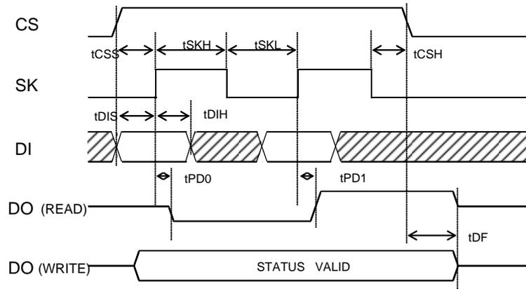
Fig.1 Sync data input / output timing diagram
