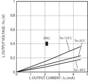
Fig.5 L output voltage  $V_{OL}$ -IOL ( $V_{CC}=4.0\text{V}$ )
