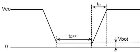
Recommended conditions of  $t_R$ ,  $t_{OFF}$ ,  $V_{bot}$
