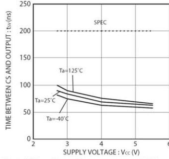
Fig.24 Time from CS to output establishment tSV
