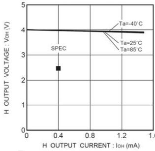
Fig.9 H output voltage  $V_{OH-IOH}$ ( $V_{CC}=4.0\text{V}$ )
