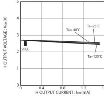
Fig.6 H output voltage  $V_{OH}$ -IOH ( $V_{CC}=2.7\text{V}$ )
