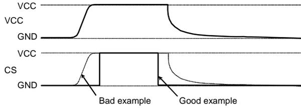
Fig.86 Timing at power ON/OFF
