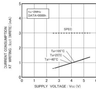
Fig.40 Current consumption at WRITE action Icc1(WRITE, fSK=2MHz)
