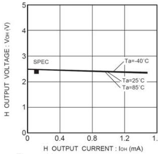
Fig.8 H output voltage  $V_{OH-IOH}$ ( $V_{CC}=2.5\text{V}$ )
