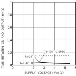
Fig.54 Time from CS to output establishment tSV
