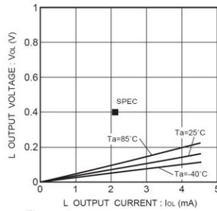
Fig.6 L output voltage  $V_{OL-IOL}$ ( $V_{CC}=4.0\text{V}$ )
