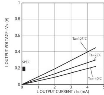
Fig.4 L output voltage  $V_{OL}$ -IOL ( $V_{CC}=2.7\text{V}$ )
