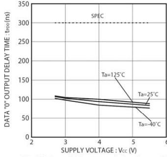
Fig.23 Data "0" output delay time tPDO
