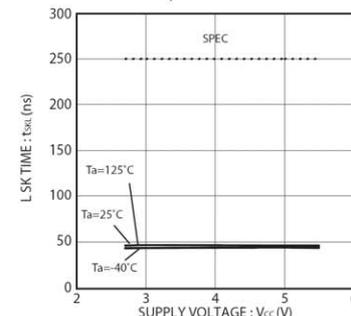
Fig.16 SK low time  $t_{SKL}$
