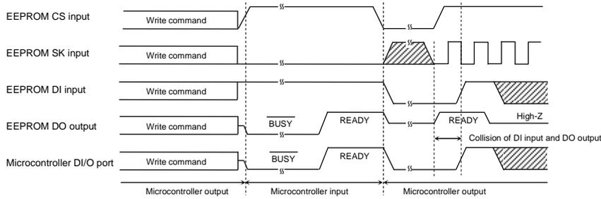
Fig.48 Collision timing at DI, DO direct connection
