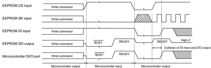
Fig.82 Collision timing at DI, DO direct connection
