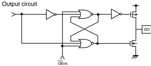
Fig.71 Output circuit (DO)
