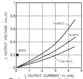
Fig.4 L output voltage  $V_{OL-IOL}$ ( $V_{CC}=1.8\text{V}$ )
