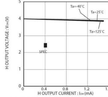
Fig.7 H output voltage  $V_{OH}$ -IOH ( $V_{CC}=4.0\text{V}$ )
