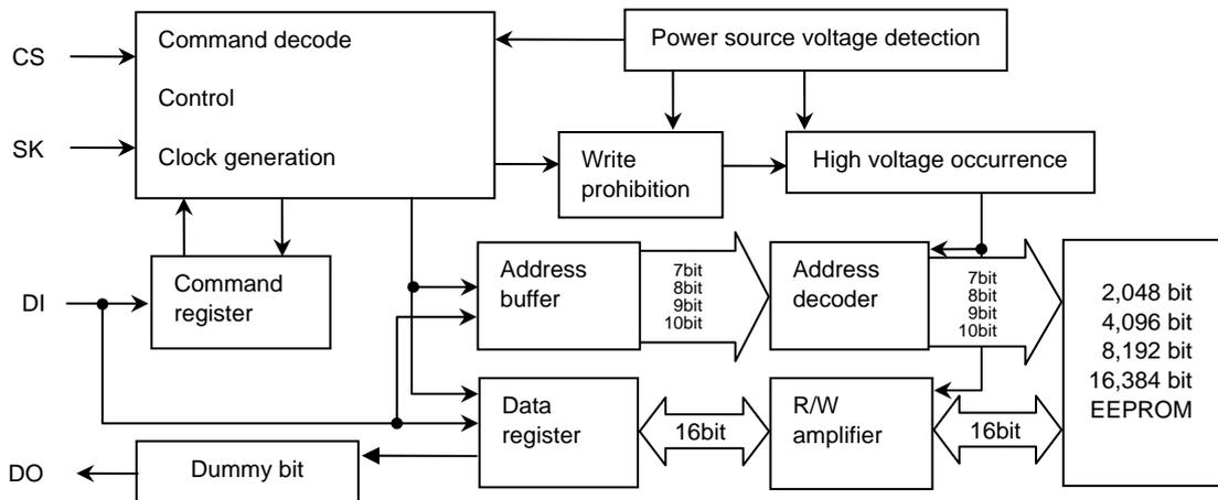
Fig. 27 Block diagram
